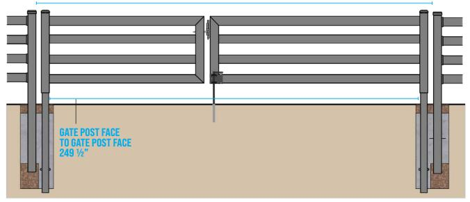
\*\*\*Gate Post Face to Gate Post Face Dimensions are reference only and rounded to the nearest  $\frac{1}{4}$ ". End Post Face to End Post Face Dimensions are exact and must be within the nearest  $\frac{1}{8}$ ".
