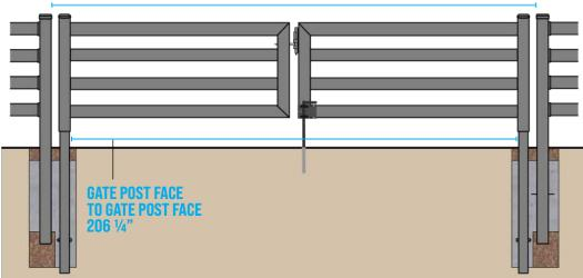
• The nominal opening between gate faces for Dual Gates is 4 ¼" when an EZ Latch is used. When not using an EZ Latch, the gap between gate faces is 3 ¼". In this case, 1" should be removed from the End Post Face to End Post Face Spacing.
