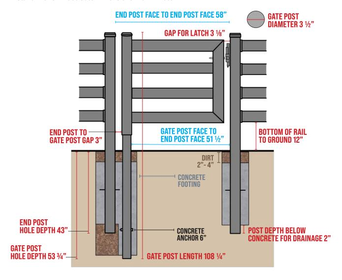
The installation dimensions for all stand alone Buckley Fence Gates are the same for all three sizes of gate, EXCEPT for the End Post Face to End Post Face measurement and the Gate Post Face to End Post Face measurement. These differentiating measurements are marked in the following figures in blue.
