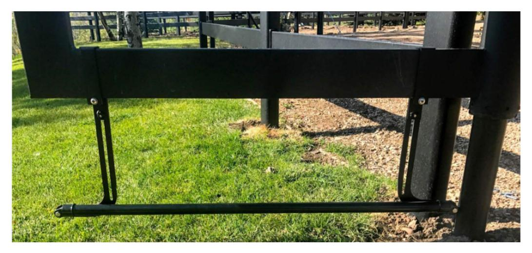
Adjust the height of the boomerang brackets by loosening the slide screws and retighten once positioned Swing the gate to assure this position works without ground interference
