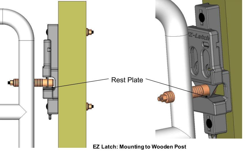
Step 1: With the pin positioned on the gate and in front of the latch post, position the latch to make contact with the pin on the rest plate as shown. With a marker make two dots at the slot centers to position the holes for the bolts.
